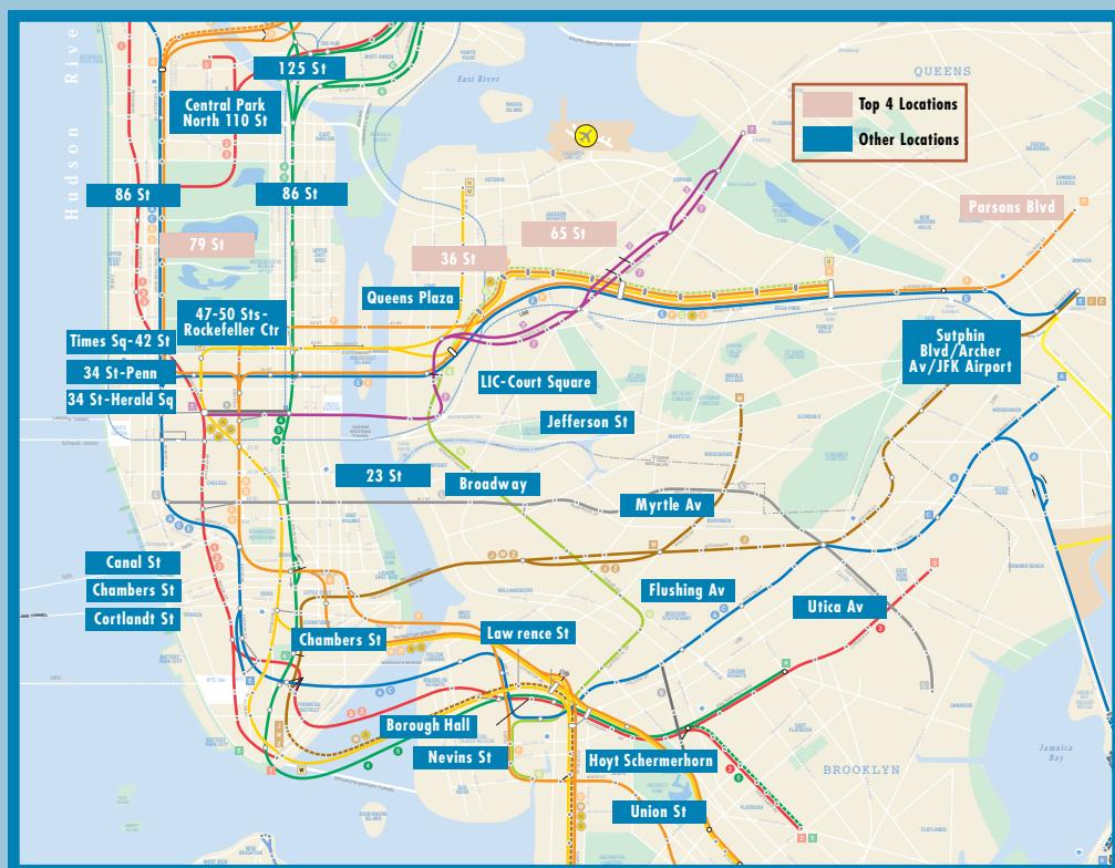
Flood-prone locations in the NYCT system and other locations where flooding or water entry into the system occurred in the past.
